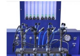
Response time (RST) of the injectors (Delphi/Denso)
