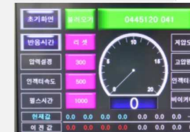
Response time (RST) of the injectors (Delphi/Denso)
